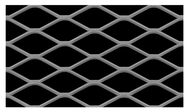
LW Pitch:50.80mmStrand Width:3.12mmSW Pitch:22.58mmThickness:3.00mmWeight:2.25 kg / m2Open Area:72%
